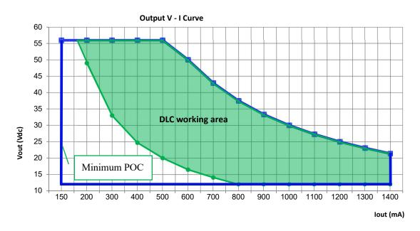
Note: When the output current is set, the output voltage is automatically limited within the curves.
